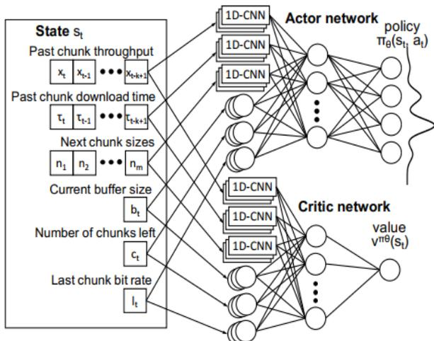
Figure 7: The Actor-Critic algorithm that Pensieve uses to generate ABR policies. [16]
