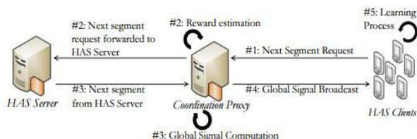
Figure 5: Logical work-flow of the proposed solution. [22]
